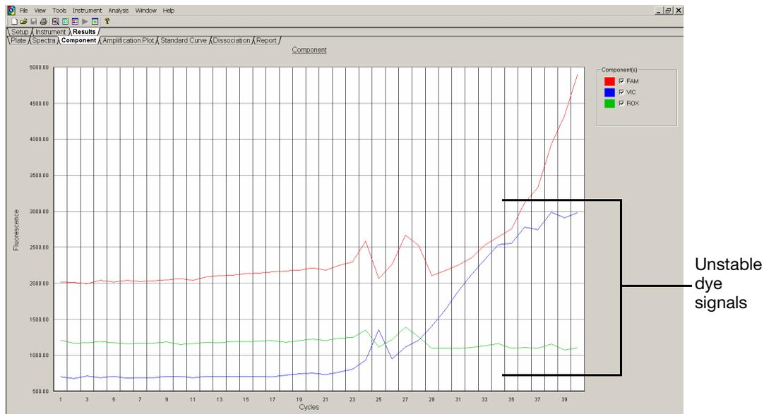
**IMPORTANT!** This signal determination *may* be implemented as a routine procedure to monitor the life of the halogen lamp. However, it is critical that the reading is taken from the *same* sample well to provide a better comparison between determinations.
