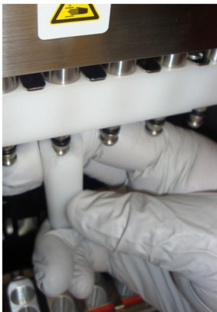
2. Using the D-ring installation tool, slip a new D-ring into the nozzle groove. Keep the flat inner surface of the D-ring in contact with the installation tool so that the D-ring does not roll. Ensure that the D-ring is placed properly on the nozzle to prevent leakage.
