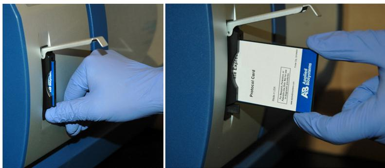
4. Insert the appropriate protocol card in the slot with the arrow pointing toward the instrument and the label facing left.
