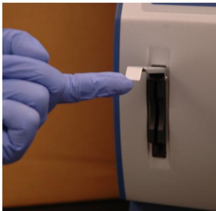
3. Insert the protocol card in the slot with the arrow pointing toward the instrument and the label facing left.
