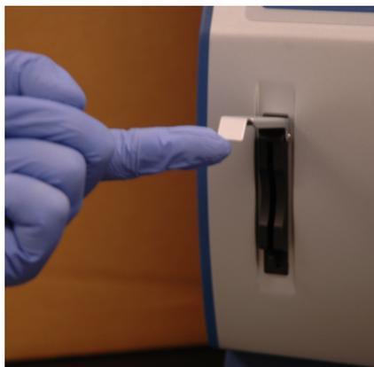
3. To remove an installed card, push the button located below the card slot (see the photo below), then pull the card out of the slot. Place the card in the plastic cover in the box. Store the card protected from light.
