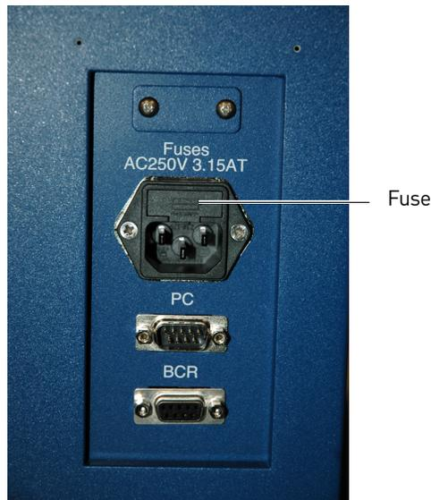
3. Pull the fuse holder out of the compartment and inspect the fuse. If the fuse is burned or there is a break in the fuse element, replace the 3.15 A fuse with the identical type fuse.
