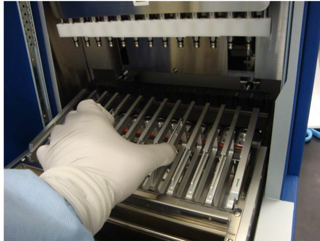
5. Insert the tip and tube rack into the instrument with row E in the front.
