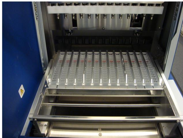
5. Using the plastics shipped with the instrument and with the AutoMate Express™ Install Kit, load the tip and tube rack in the following order:
