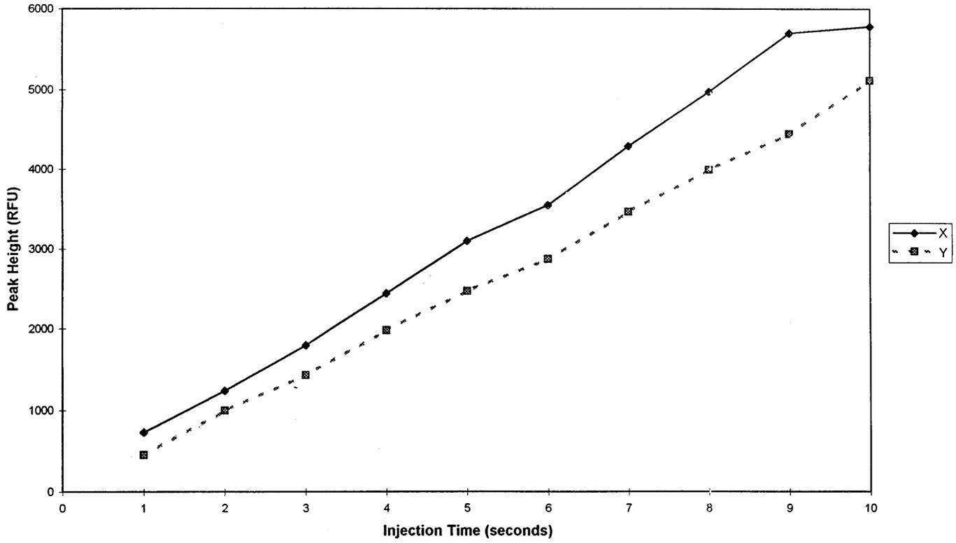
FIG. 2a—Injection time vs. X and Y peak heights.
