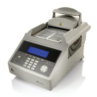
The Dual 96-Well GeneAmp® PCR System 9700 is a complete system that includes the base and sample block module.
