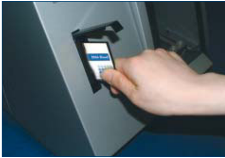
Figure 1 Inserting an EZ1 Card, containing protocols, into the BioRobot EZ1.
