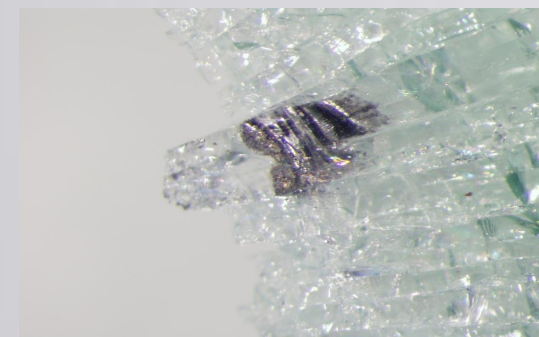
Microscopic lead metal transfer
