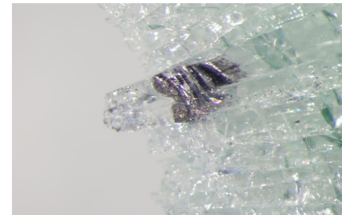
Microscopic lead metal transfer
