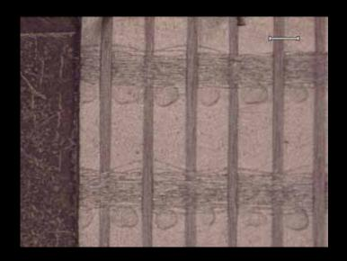
View of underside of a duct tape film; adhesive and scrim removed showing the fabric imprint in the tie coat.
