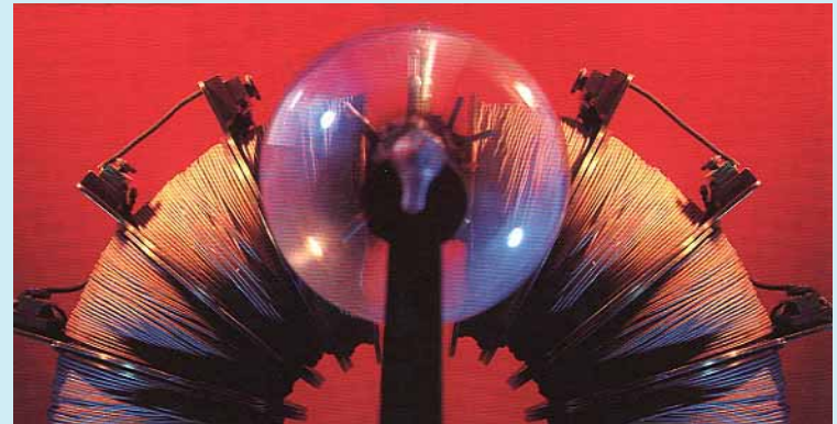
Aston's original "Positive-Ray Mass Spectrograph"
