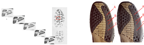
Progression of general wear on one outsole element from new (A) 5 months of general wear on an outsole to approximately 150 miles of use 4 months later (E).
