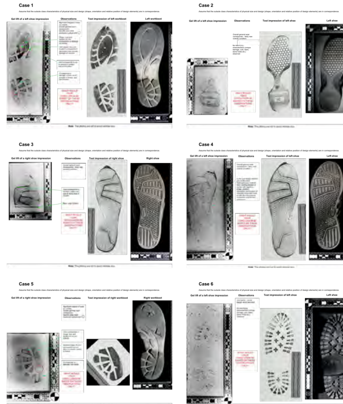
Figure 1. Six sets of photographs, representing six fabricated crime scenes, were prepared and disseminated via e-mail to IAI certified footwear examiners and students enrolled in the University of Strathclyde's 2008-2009 Master of Science – Forensic Science programme. Each set consisted of a gelatin lift of an unknown impression, a scanned image of a test impression and photographs of the suspect shoe. The colour of the gelatin lifts was inverted and both the gelatin lifts and the outsole photographs were horizontally flipped in Adobe Photoshop. All characteristics and observations to be considered in the comparison were labelled for each impression. The examiners were to assume that all observations listed were correct. It was not expected that they conduct their own comparison, rather that they assess each comparison set as described and choose the SWGTEAD conclusion that best matched their opinion. We do recognize that there are several other ways in which to express conclusions when reporting footwear results; however, we chose the SWGTEAD guidelines as an example of standardized terminology. When reporting a final conclusion, the examiners were requested to only use the provided expressions, even if they do not typically use this terminology in their own reports.
