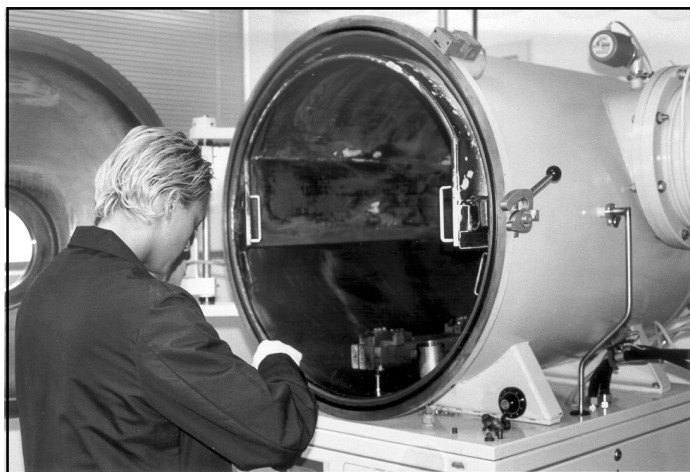
Forensic Scientist Linda Engstrom uses the vacuum metal deposition chamber to develop latent prints.
