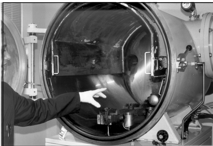
Forensic Scientist Linda Engstrom uses the vacuum metal deposition chamber to develop latent prints.
